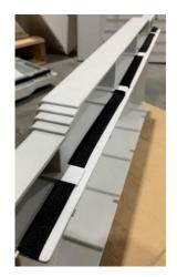
**<u>Step 5: Final sealing</u>** – final sealing is to be done on the top and bottom panel.
