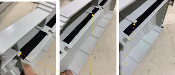
Cut out tabs as shown to allow for full sealing
